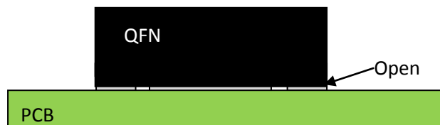
Figure 6 Illustration of solid solder paste pattern in die-paddle causing QFN lifting and open connections
