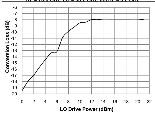
Low Band Mixer: Conversion Loss vs. LO Driver Power RF = 73.6 GHz, LO = 35.2 GHz, and IF = 3.2 GHz
